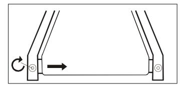
walking/running characteristics. Some users will affect tracking differently. Expect to make adjustments as required to center the treadbelt. Adjustments will become less of a maintenance concern as the belt is used. Proper belt tracking is an owner responsibility common with all treadmills.
